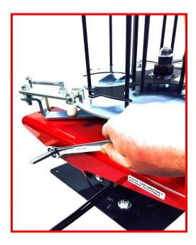
**Step 16** – The pull cord or optional radio release can now be connected to the machine.
