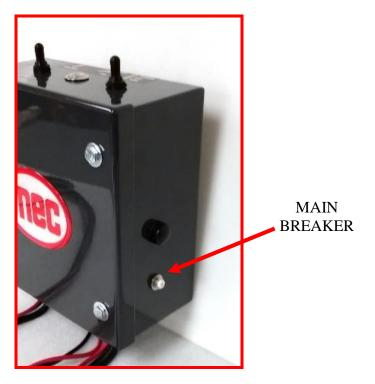
**Elevation Toggle Switch** - Pushing the switch downward will turn the elevation motor on. Note that the elevation motor will randomly start/stop when the machine is in operation. This prevents shooters from being able to predict the direction of the next target. Pushing the toggle switch upward allows you to nudge the elevation motor which elevates the machine up and down enabling you to check the clays flight.
