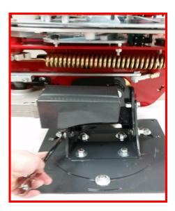
**Step 10 –** Rotate the machine by loosening the three 1/2" nuts. Once the machine is rotated to desired position, retighten the three nuts to secure machine.
